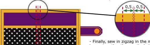
Finally, sew in zigzag in the middle to keep the two leaves together then vertical stitches 0,5 cm from the middle.
